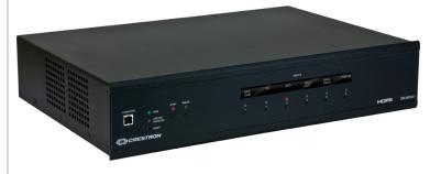
switching latency that plagues typical HDMI switchers. QuickSwitch HD achieves very fast switching of HDMI signals by maintaining a constant HDCP connection with each HDMI device in the system, eliminating the need to re-authenticate each time a different source is selected.
